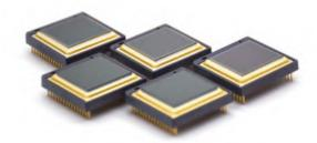
Holo HP13 is equiped with new ceramic encapsulated detector, which are lighter, lower power consumption and last longer.
